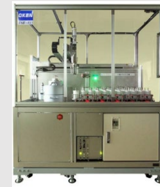
Food Inspection Monitor With Sample Changer Trace Radioactivity Measurement Device
